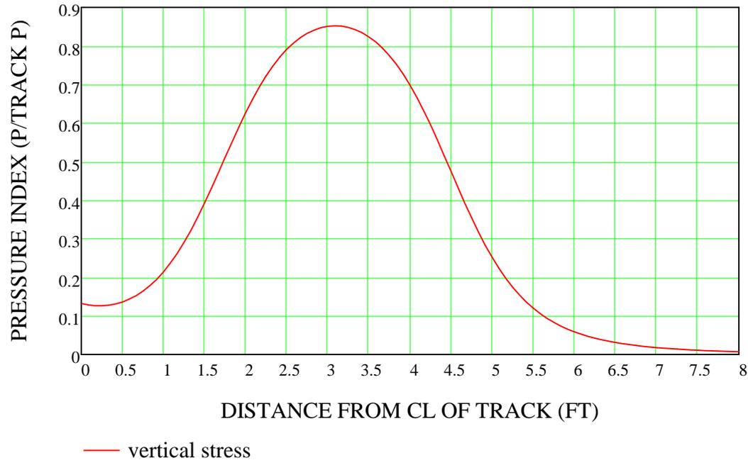
showing the overlap of the stress bulbs under the machine.
